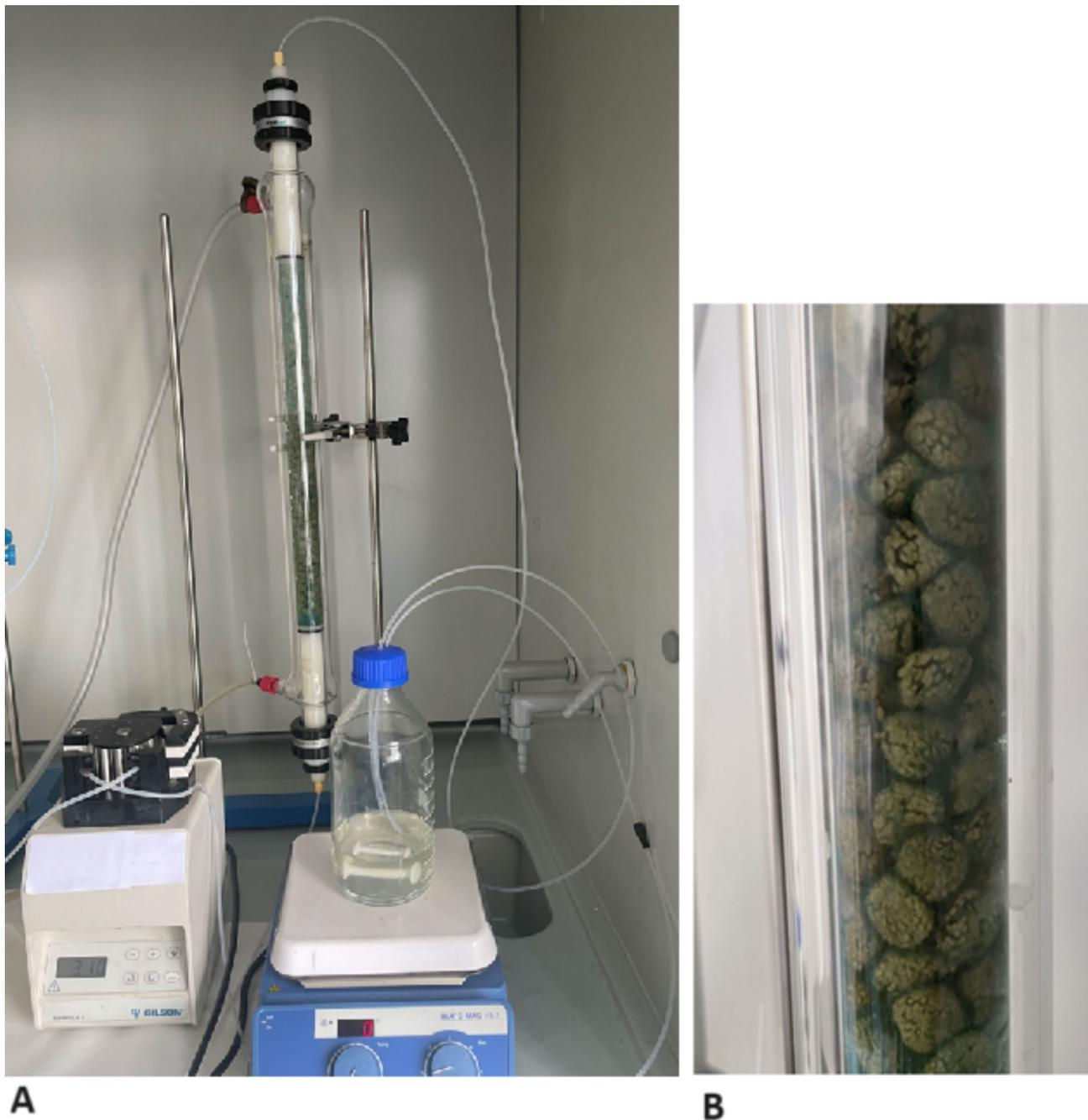
**Fig. 3** COS production system: **(A)** PBR with equipment (peristaltic pump, magnetic stirrer). The column is connected to a thermostat (not visible in the photo), **(B)** PUF-immobilized mycelium in the column reactor
